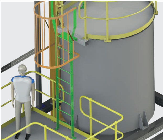
CAGED LADDER FROM PLATFORM TO TOP OF TANK
